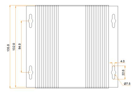
Tolerance: ±0.3 Unit: mm
